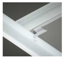
This is a hook-over bracket supplied fixed to the upstand of the panel. Access is obtained by pushing up the opposite end of the panel and sliding back. This reveals the flange which can then be lowered to a vertical position (lift & tilt).
