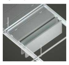
This integral feature allows tiles to be hung vertically from C-Profiles which provides unobstructed ceiling void access. Complete panel runs can be hung together during maintenance without causing damage to the tile.
