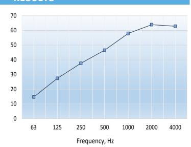
Single figure rating:  $D_{n,c,w}(C;Ctr) = 48 (-2;-7) dB$  According to BS EN ISO 717-1: 1997
