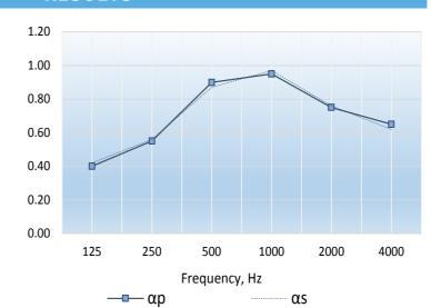
Single figure rating :  $\Omega \omega$  0.75 In accordance with BS EN ISO 11654: 1997
