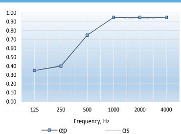
Single figure rating :  $\Omega_{\odot}$  0.70(MH) In accordance with BS EN ISO 11654: 1997
