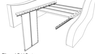
**SAS205** is a hook-on corridor suspended steel ceiling system; to facilitate access tiles are suspended at the perimeters using brackets and closure angles. A range of acoustic backing options provide up to 49dB acoustic attenuation or Class A acoustic absorption. For further details please visit <a href="https://sasintgroup.com/metal-ceilings/suspended-sas205/">https://sasintgroup.com/metal-ceilings/suspended-sas205/</a>
